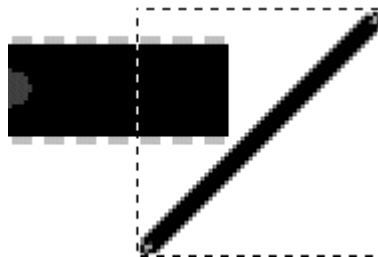
Figure 5: A diagonal wire, its influence on the mouse and how it may interfere with a component
